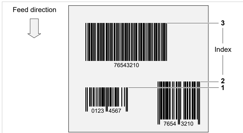
Fig. 19: The indexing of the bar codes is done in the order of the bar code top edges on the label in feed direction.
